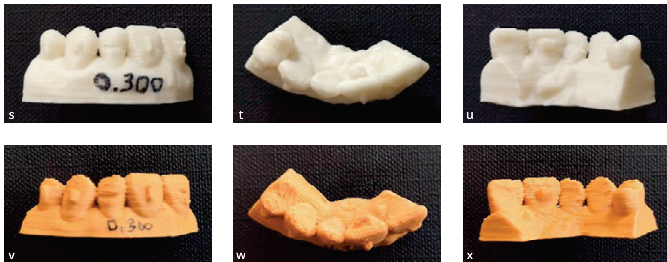
Figs 2a to x Sectioned maxillary dental model: (a to c) STL master file; (d to f) DLP control model (layer height 20.0 \mu\text{m} ); (g to i) Lignin-based model (layer height 50.0 \mu\text{m} ); (j to l) Polylactide model (layer height 50.0 \mu\text{m} ); (m to o) Lignin-based model (layer height 150.0 \mu\text{m} ); (p to r) Polylactide model (layer height 150.0 \mu\text{m} ); (s to u) Lignin-based model (layer height 300.0 \mu\text{m} ); (v to x) Polylactide model (layer height 300.0 \mu\text{m} ).
