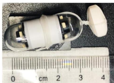
Fig. 10. Capsule endoscopic method for visualization of the behavior of solid dosage forms in the gastrointestinal tract (reprinted with permission from Blaabjerg et al. [116]).
