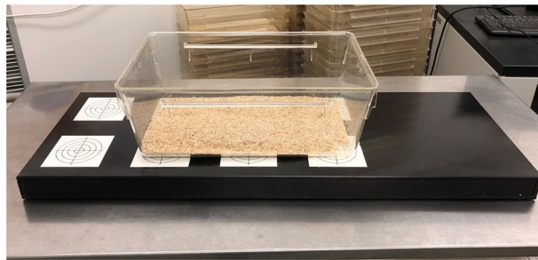
Figure 1. Overview of the radio telemetry tracking system. The radio telemetry platform is made up of eight antennas generating electromagnetic fields. A polycarbonate cage is placed on top of it.
