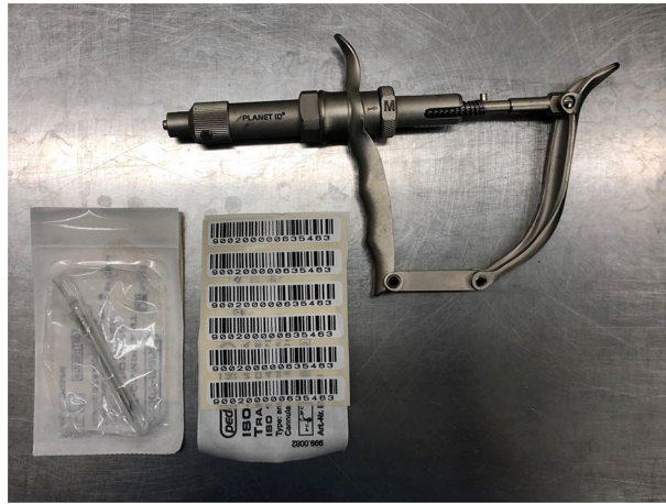
Figure 2. RFID Injection gun. Injection gun with a special needle containing the coded RFID which is implanted in the mice's subcutis.
