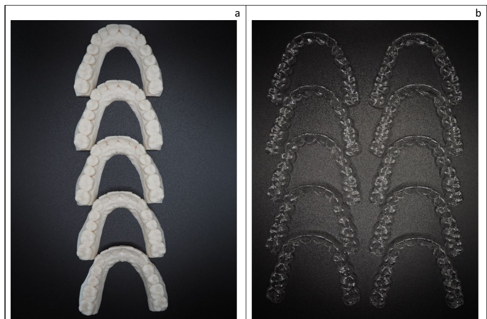
Fig. 1 FFF-printed models with planned sequence step of 0.1 mm distalization at different layer heights and their corresponding aligners. a FFF models with different layer heights arranged from top to bottom: 100 \mu\text{m} , 150 \mu\text{m} , 200 \mu\text{m} , 250 \mu\text{m} , 300 \mu\text{m} . b Corresponding aligners arranged from up to bottom: 100 \mu\text{m} , 150 \mu\text{m} , 200 \mu\text{m} , 250 \mu\text{m} , 300 \mu\text{m} layer height; on the left 0.5 mm aligner series, on the right: 0.75 mm aligner series
