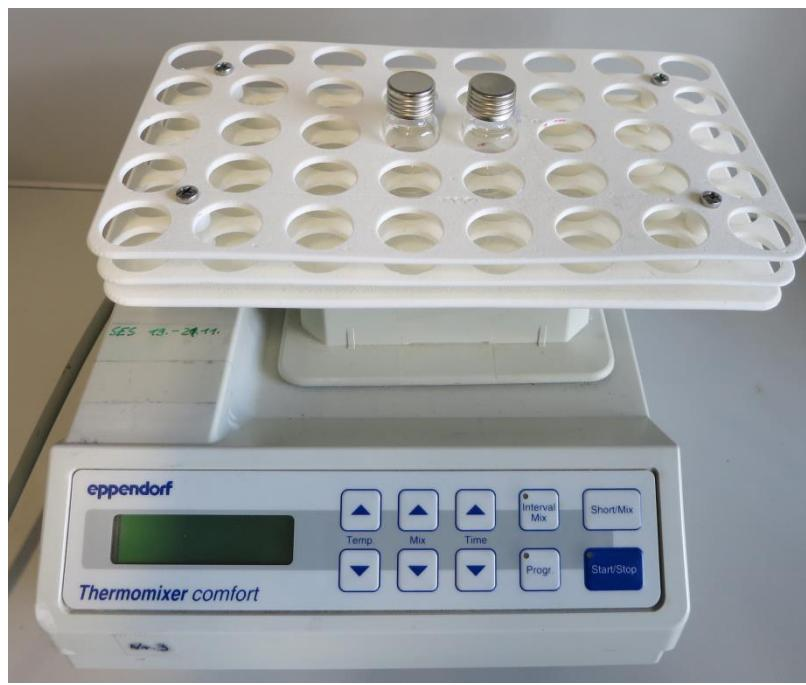
**Figure S2.** Adapter for the Eppendorf shaker that was used for the biocatalysis reactions performed at a larger scale.
