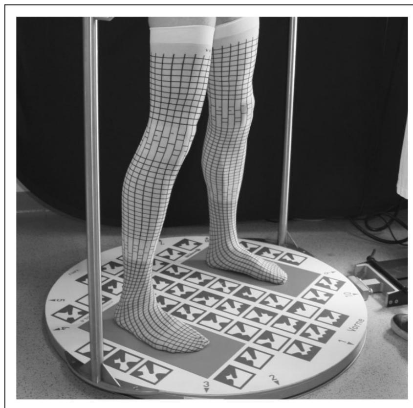
**Figure 2.** Measuring volume with the Image3D® system.
