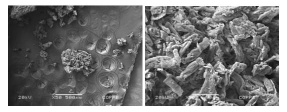
Figure S7: SEM analysis of cellulose functionalized with Glymo. Experimental Conditions: 1 mg sample metallized by gold under vacuum, analysed in a Zeiss EVO® 50H microscopy.
