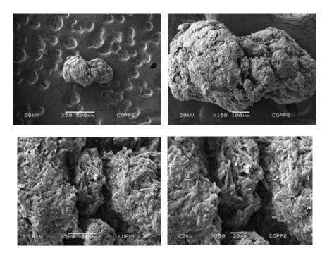
Figure S8: SEM analysis of Glymo functionalized cellulose with Cal-B. Experimental Conditions: 1 mg sample metallized by gold under vacuum, analysed in a Zeiss EVO® 50H microscopy.
