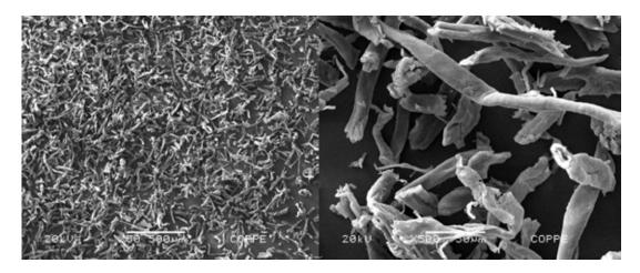
Figure S3: SEM analysis of celullose. Experimental Conditions: 1 mg sample metallized by gold under vacuum, analysed in a Zeiss EVO® 50H microscopy.
