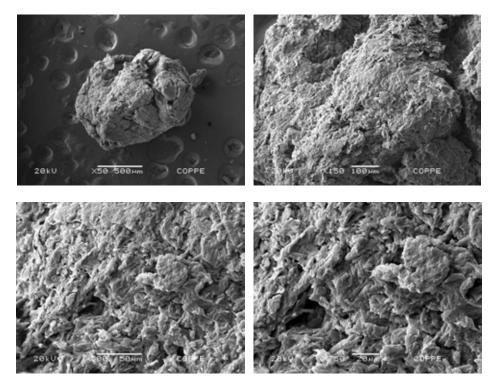
Figure S9: SEM analysis of Glymo functionalized cellulose with transaminase. Experimental Conditions: 1 mg sample metallized by gold under vacuum, analysed in a Zeiss EVO® 50H microscopy.
