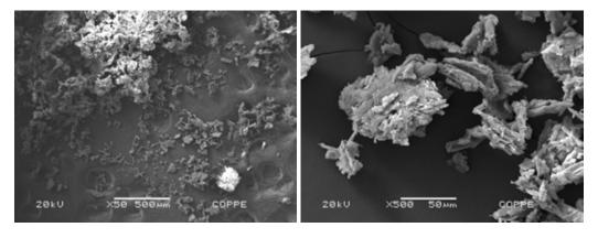
Figure S4: SEM analysis of APTES functionalized celullose. Experimental Conditions: 1 mg sample metallized by gold under vacuum, analysed in a Zeiss EVO® 50H microscopy.
