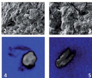
Fig. 1 Confocal Laser Scanning Microscopy (CLSM) and Scanning Electron Microscopy (SEM) analysis of ECel-VF and GCel-VF. (1) SEM analysis of cellulose before functionalization; (2) SEM analysis of ECel-VF; (3) SEM analysis of GCel-VF; (4) CLMS analysis of ECel-VF; (5) CLMS analysis of GCel-VF.
