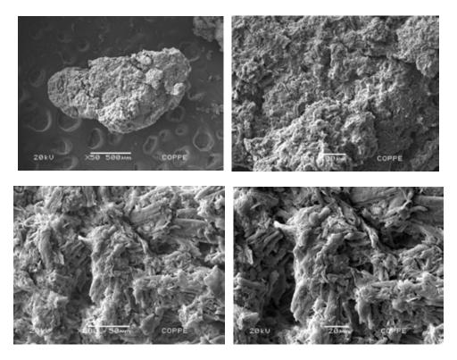
Figure S10: SEM analysis of glutaraldehyde-functionalized cellulose with transaminase. Experimental Conditions: 1 mg sample metallized by gold under vacuum, analysed in a Zeiss  $EVO^{@}~50H~microscopy.$
