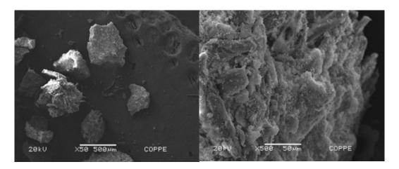
Figure S5: SEM analysis of APTES + glutaraldehyde functionalized celullose. Experimental Conditions: 1 mg sample metallized by gold under vacuum, analysed in a Zeiss EVO® 50H microscopy.
