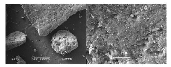
Figure S6: SEM analysis of Cal-B immobilized on glutaraldehyde functionalized cellulose. Experimental Conditions: 1 mg sample metallized by gold under vacuum, analysed in a Zeiss EVO® 50H microscopy.
