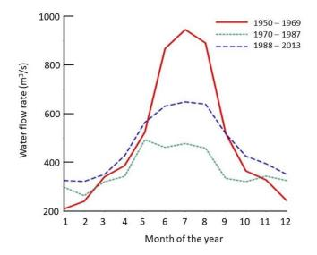
**Figure 2.** Average monthly water flows as measured at the Kapchagai hydropost during three periods of time: immediately prior to closure of the dam (1950–1969), while the reservoir was being filled (1970–1987), and after filling of the reservoir ceased (1988–2013). Raw data are from Kazhydromet.
