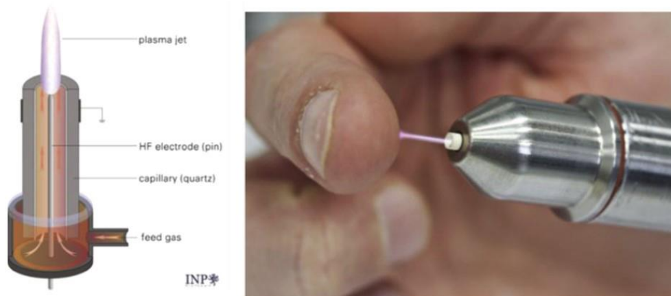
Figure 1.10 Atmospheric pressure plasma jet kINPen MED. Physical structure and application on skin. The figure is adapted from Bekeschus et al. [151].
