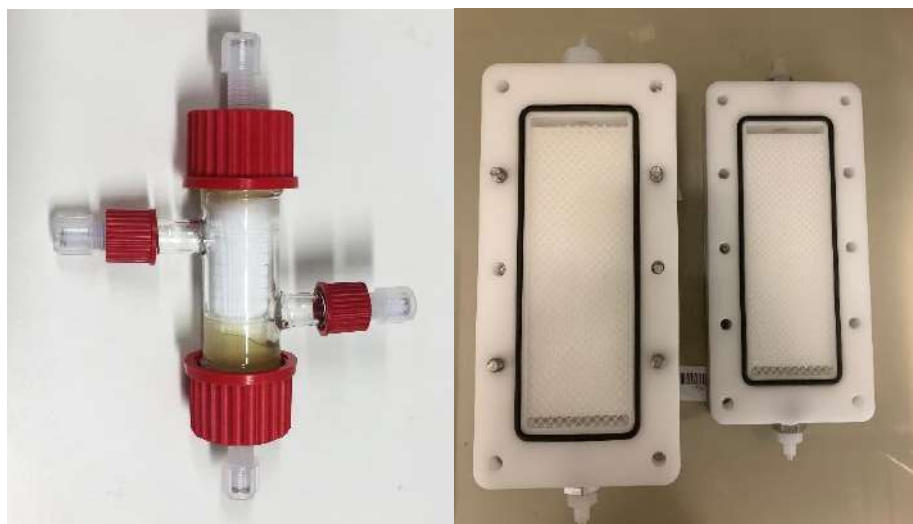
Figure S4. Hollow fiber (HF) contactor with modified housing and the flat sheet (FS) membrane contactor.
