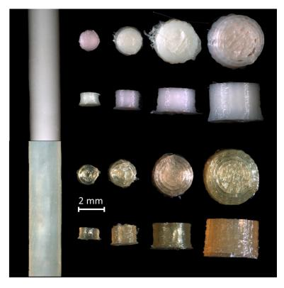
**Figure 2.** Microscopic images of the filaments and printed tablets with hyprolose (HPC) as polymer (top row: containing caffeine; bottom row: containing propranolol hydrochloride; from left to right: filament, mini tablet diameter 1.5, 2.0, 3.0, and 4.0 mm).
