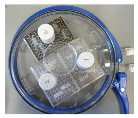
**Figure 2.** Image of compressed plates within the hypoxic chamber. Weights of 1000 g were placed on top of the self-constructed compression lids to apply a force of 9.81 N to an area of 0.079 cm<sup>2</sup> per well.
