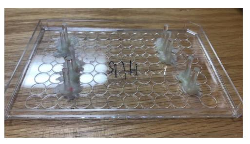
**Figure 3.** Image of the compression device. Plastic rods with 16 mm length and 3.175 mm diameter were fixed onto a lid of a 96-well plate.
