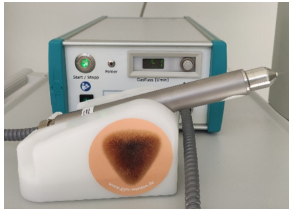
Figure 1. The Kinpen Med medical argon plasma device (Neoplas Tools, Greifswald, Germany) was used to generate non-invasive physical plasma (NIPP).
