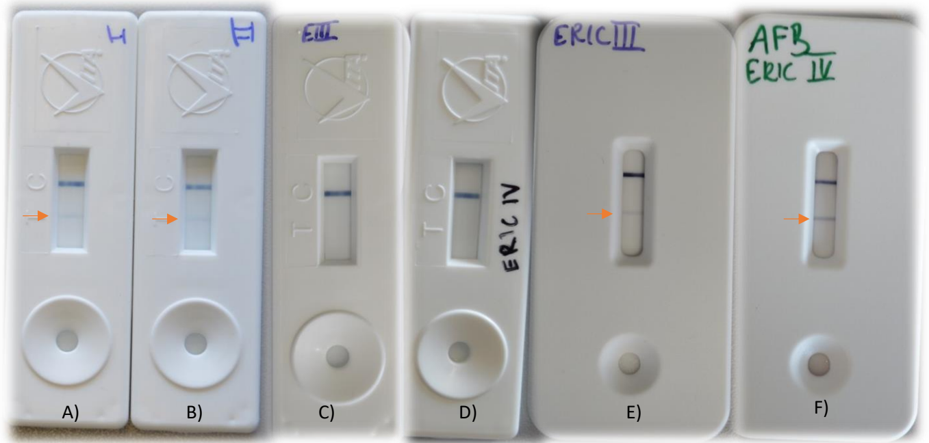
Figure 56 LFD comparison of commercially available AFB-LFD (Vita) and developed AFB-LFD (Senova)
