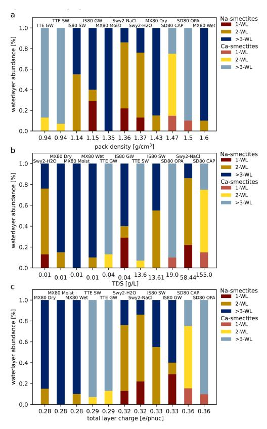
**Figure 7.** Summary of the number of water layers developed in hydrated bentonite samples studied by wet-cell X-ray diffractometry [9,22,30]. (a) water uptake verses packing density, (b) water uptake verses total dissolved solids (TDS), (c) water uptake verse total layer charge.
