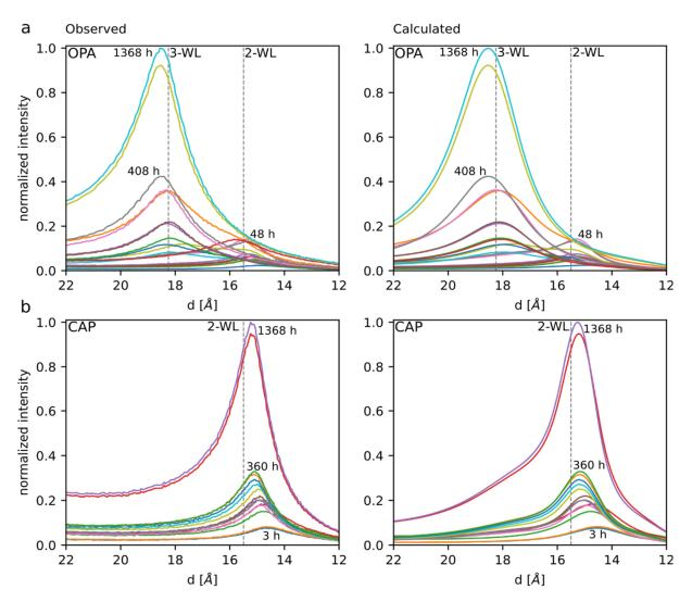
**Figure 4.** Comparison between observed and calculated XRD patterns for the varying hydration states of Milos bentonite. (**a**) SD80 infiltrated by Opalinus clay pore water, and (**b**) SD80 infiltrated by diluted cap rock brine.
