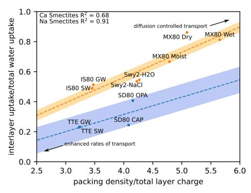
**Figure 8.** Plot showing the correlative relationships between the interlayer/total water uptake ratio versus the packing density/total layer charge ratios for Ca-(blue) and Na-(orange) bentonites (data source given in Table 3). The shaded areas correspond to the standard deviation of the data sets.
