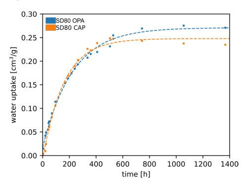
**Figure 2.** Comparison of the inflow of solution into the SD80 bentonite with Opalinus clay pore water (OPA), and diluted cap rock brine (CAP). Volumes were calculated from weight measurements after correction for salt content.
