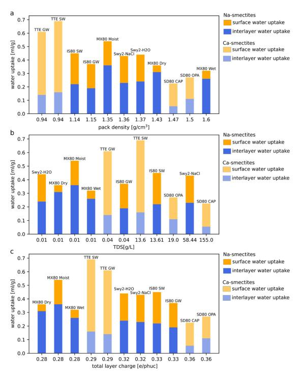
**Figure 6.** Summary of the amounts of interlayer and non-interlayer water in hydrated bentonite samples studied by wet-cell X-ray diffractometry [9,22,30]. (a) water uptake verses packing density, (b)water uptake verses total dissolved solids (TDS), (c) water uptake verse total layer charge.
