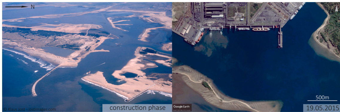
Fig. 13. Left: Historical aerial image of Richards Bay Harbour during construction (© Klaus Jost – jostimages.com). Intensive sand (light brownish areas) relocation occurred during construction. The majority of sand features were temporary and do not exist today. Note that North is to the right. Right: Resuspension of surface sediment via berthing procedures at SB-II (source Google Earth). Sediment clouds – caused by propellers near to the seafloor – are often visible on aerial images.
