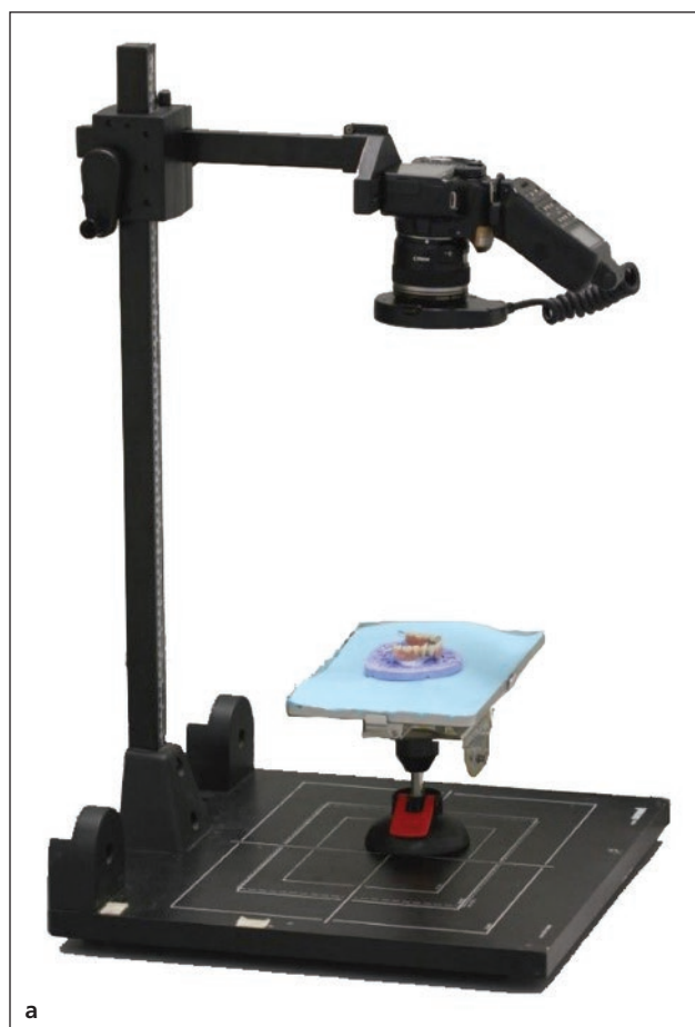
Fig 1 (a) Test set-up and (b) denture after fixation on the silicone key on the 45-degree tilted base.
