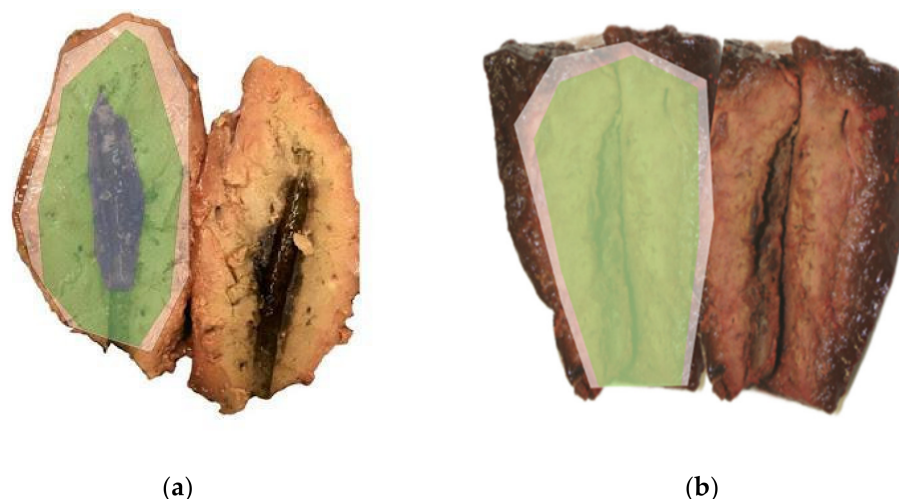
Figure 2. Cross section of the ablation zones in (a) the stand-alone applicator (25 W; 10 min) and (b) the spacer-supported applicator (25 W; 25 min). Black overlay: carbonisation zone. Green overlay: non-viable tissue. White overlay: total ablation zone (“red zone”).
