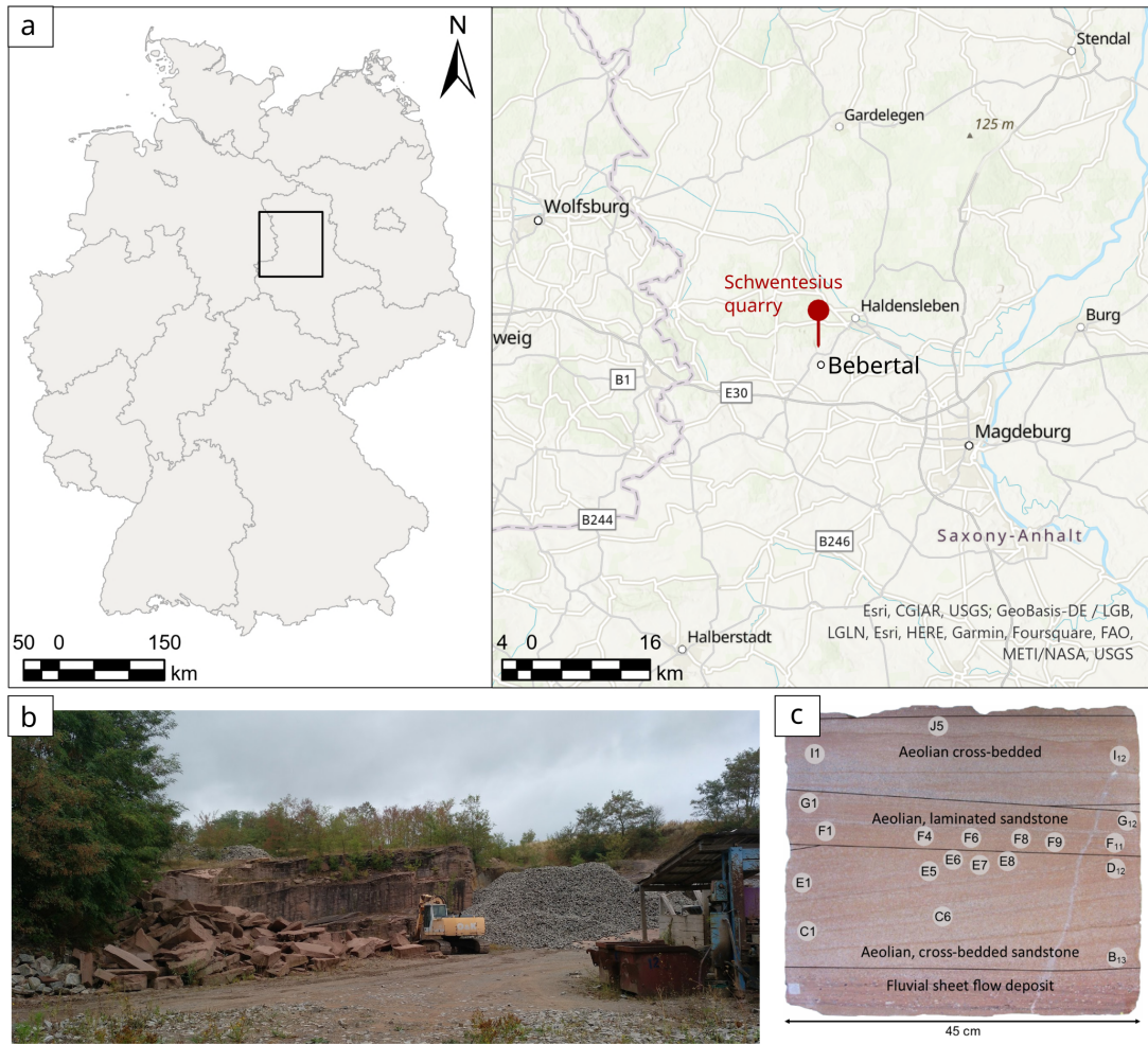
Figure 3: (a) Map of Germany with the location of the Schwentesius quarry near Bebertal. (b) Photograph of the Schwentesius quarry. (c) Sample block of the Bebertal sandstone used in the ResKin project.
