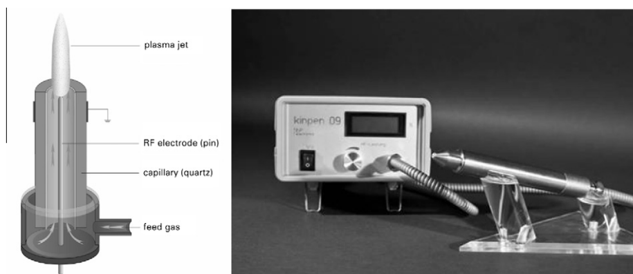
Fig. 1. Schematic (left) and photo (right) of the plasma source kINPen09.
