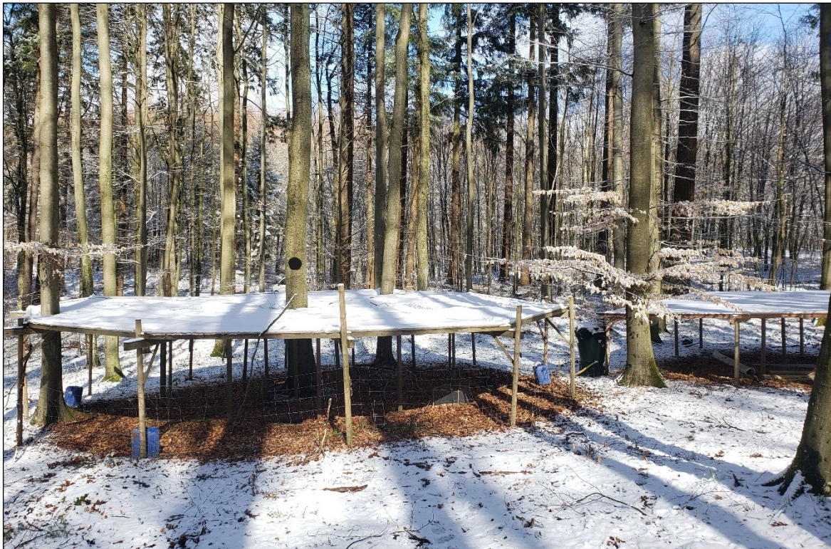
Fig. A1 Experimental setup (RnoS) at the coldest site KA, during a snow event. The rain collection roof is positioned at the back right, and the snow-out shelter is at the front left.
