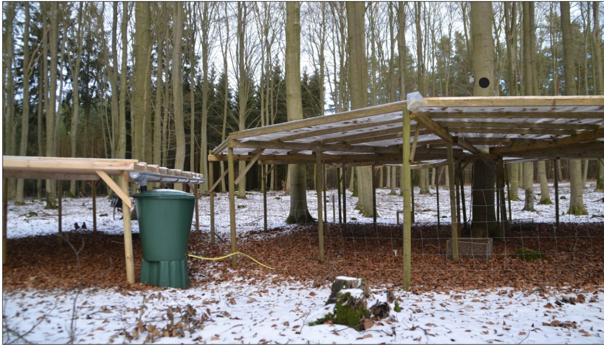
Fig. A.1. Visual impression of the experimental construction (RnoS) with the rain collection roof to the left and the snow-out shelter to the right. The target tree is marked with a black dot.
