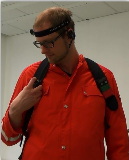
Figure 5: Powering on the LiveCity camera by pressing the black button on the right strap
