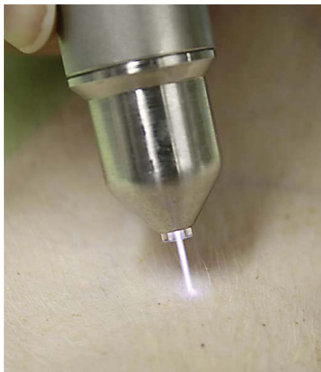
Fig. 1. Application of the plasma jet to the skin surface.
