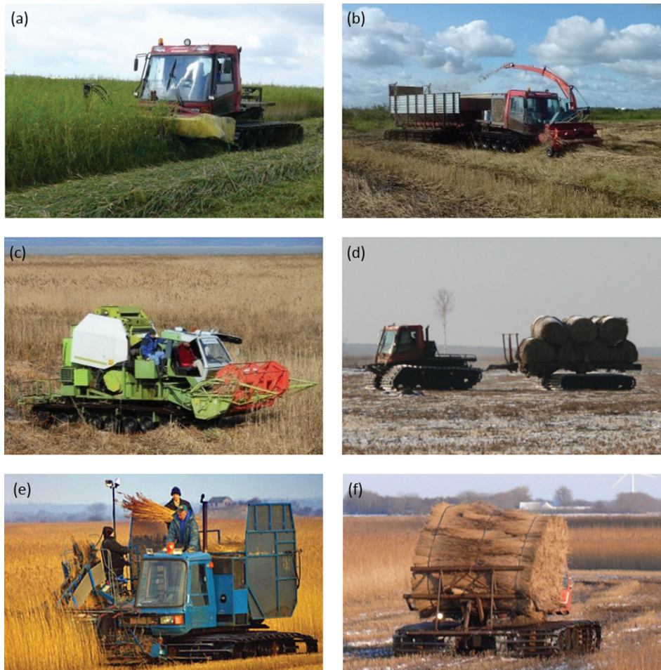
Fig. 1. Tracked machinery with low ground pressure and equipped with special devices to harvest (a and b) finely chopped biomass for biogas production, (c and d) round bales for direct combustion, and (e and f) bundles for thatching (author's photos, except (c) J. Krail, (d) I. Mirowski, and (e) Bahnsen-Clausen GbR).
