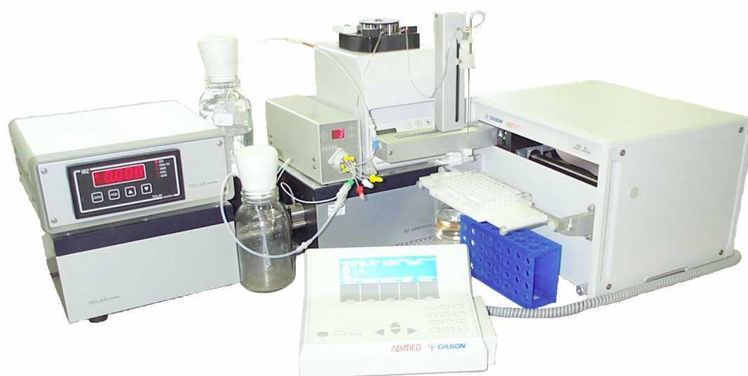
Figure 28. POLARmonitor setup with 300 µl stainless cuvette (behind waste bottle), motor driven valve, peristaltic pump, liquid handler and keypad (from left to right).
