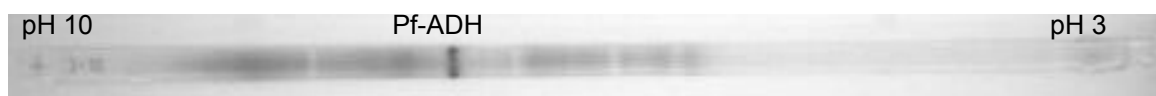
Figure 10. Isoelectric focussing gel strip (linear pH 3-10) after enzyme activity staining using racemic \alpha -phenyl ethanol as substrate.
